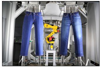
Jeanologia, the leaders in sustainable and ecoefficient technology development, launched the Handman a new technology that revolutionizes the jeans industry allowing it to reach the next level thanks to automation
